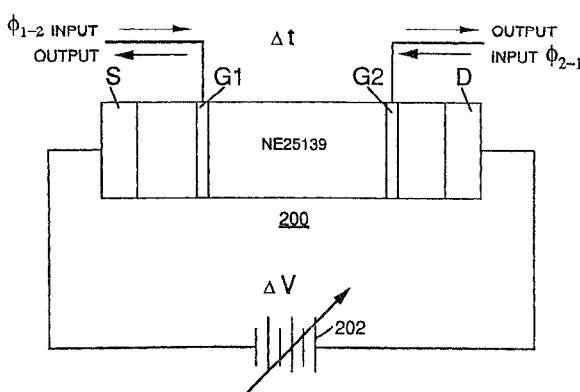
**Abstract**—An optical transmitter having a Mach-Zehnder optical modulator comprising a signal electrode fed with a driving signal for effecting modulation and a bias electrode for operating point control. Because the signal electrode and the bias electrode are independent of each other, a driving circuit and the signal electrode can be connected in a dc setup. This permits stable operating point control and improves waveform characteristics.
